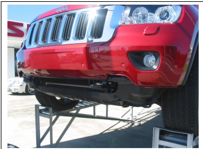
Figure 3: Bumper with lower section fully removed.
