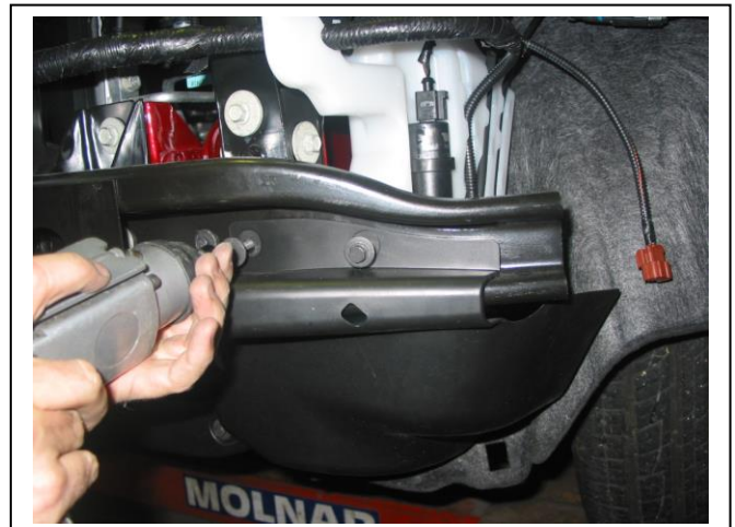
Figure 4: Remove two bolts from top and one from under side of plastic trim
